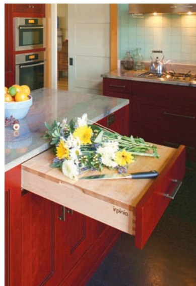
The kitchen was designed with many drawers for easy access, including refrigerator drawers in the island (not shown here). The corner drawers above are easy to access from both sides and provide incredible storage. A reinforced pull-out cutting board offers the option of sitting while working in the prep area.
